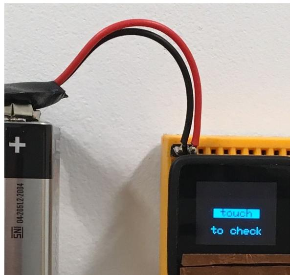
The header may be pulled, gently, by its wires, to disconnect, as shown on the right.
